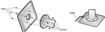
The included screw bolts can be used for attaching stands with mounting plates up to 4 mm in thickness. For stands with mounting plates thicker than 4 mm, please prepare longer screw bolts as required.
