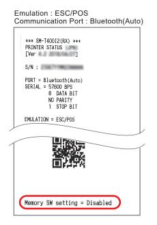
\* When the above steps 1 to 4 are performed while the setting change by memory switch is disabled, the printer prints out "Memory SW setting = Enabled" and the setting change by memory switch is disabled.
