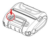
2. To put the printer into Memory Switch Setting mode, press and hold both the POWER & FEED buttons for 3 seconds. After the ERROR LED flashes five (5) times, you can configure the settings. Release the buttons after you surely confirm the LED flashes five (5) times, to get a printer into the setting mode.
